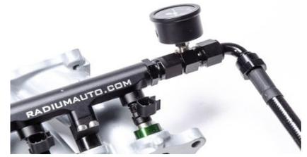
Alternatively, a pressure gauge can be installed on one of the bottom ports using a combination of NPT fittings as shown.
